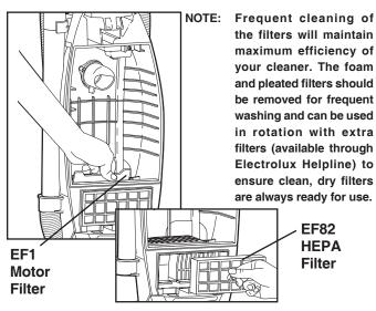
Shake filter to remove excess dust. If necessary, the filters may be cleaned by vacuuming with another cleaner.
